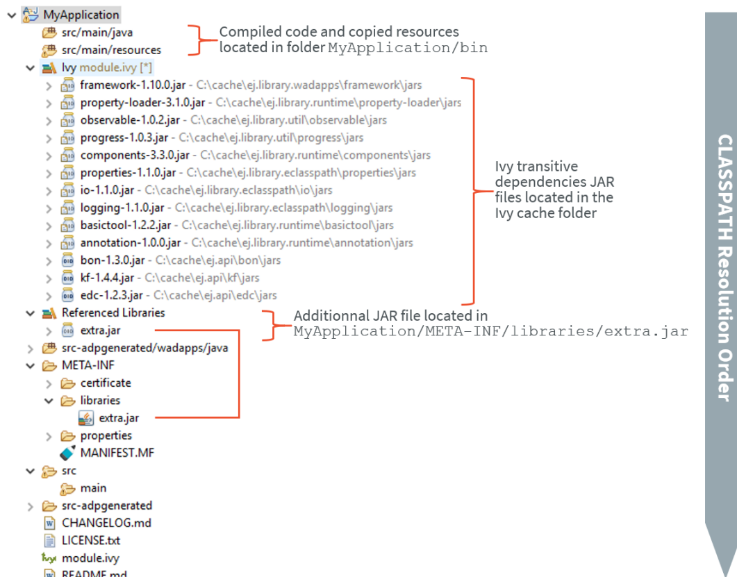
Fig. 22: MicroEJ Application Classpath Mapping
