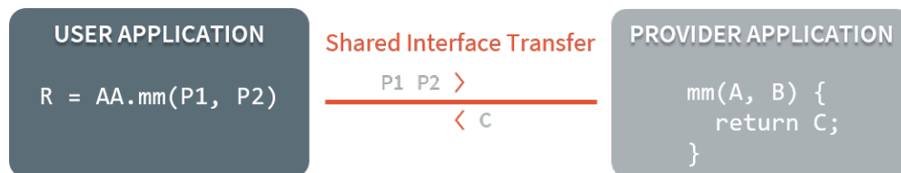
Fig. 17: Shared Interface Parameters Transfer
