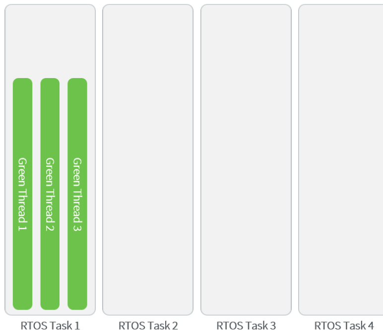
Fig. 18: A Green Threads Architecture Example
