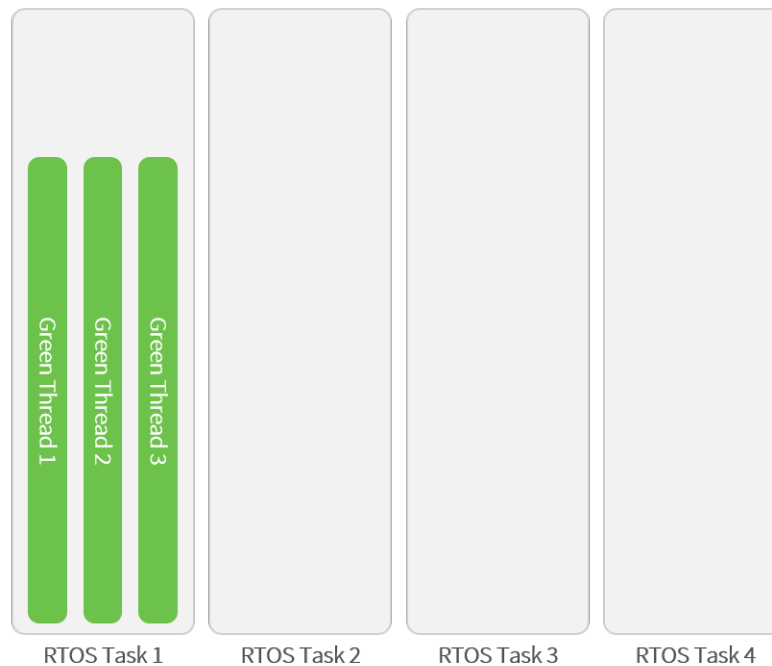
Fig. 15: A Green Threads Architecture Example
