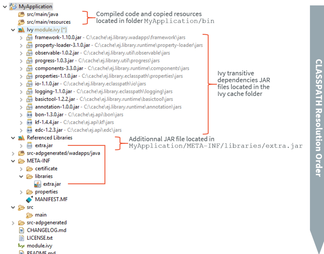
Fig. 23: MicroEJ Application Classpath Mapping
