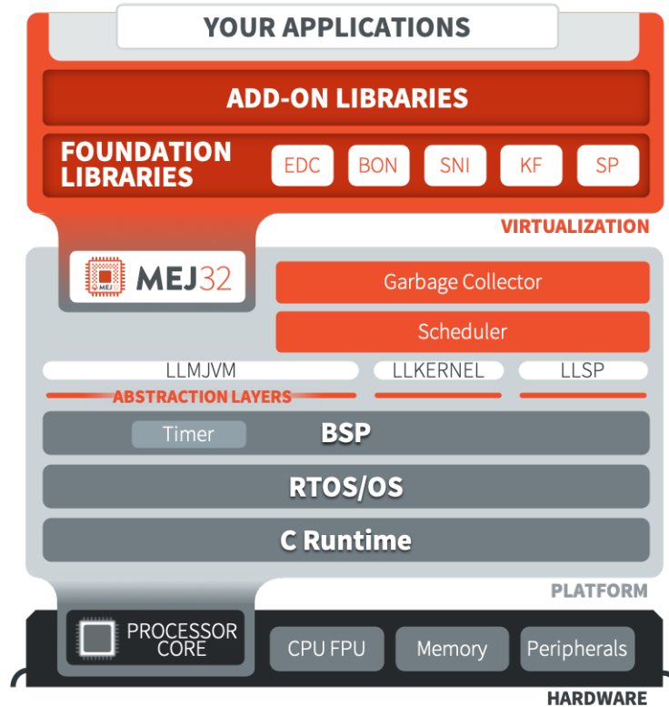
Fig. 7: MicroEJ Architecture Modules
