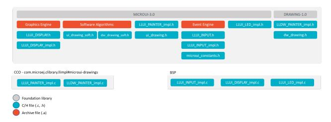
Fig. 33: MicroUI Embedded Low Level API
