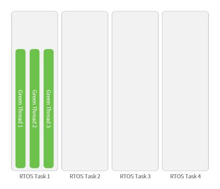
Fig. 18: A Green Threads Architecture Example
