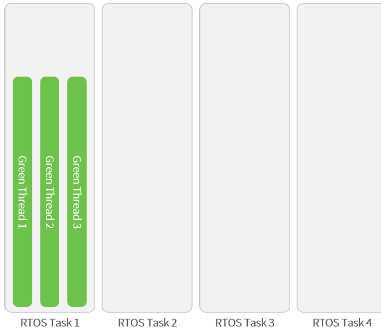
Fig. 18: A Green Threads Architecture Example
