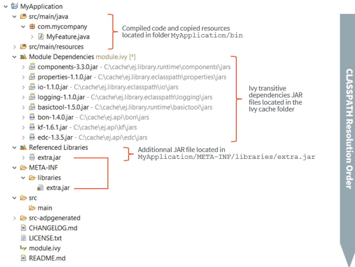
Fig. 29: MicroEJ Application Classpath Mapping
