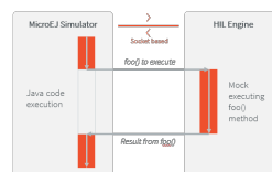
Fig. 59: The MicroEJ Simulator Executes a Native Java Method foo() .
