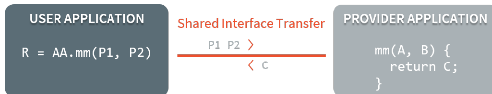
Fig. 17: Shared Interface Parameters Transfer
