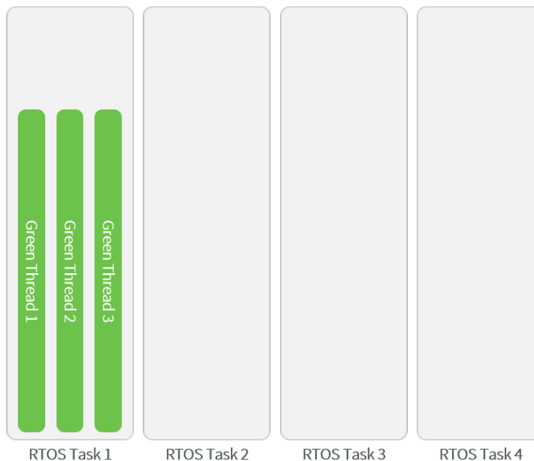
Fig. 18: A Green Threads Architecture Example
