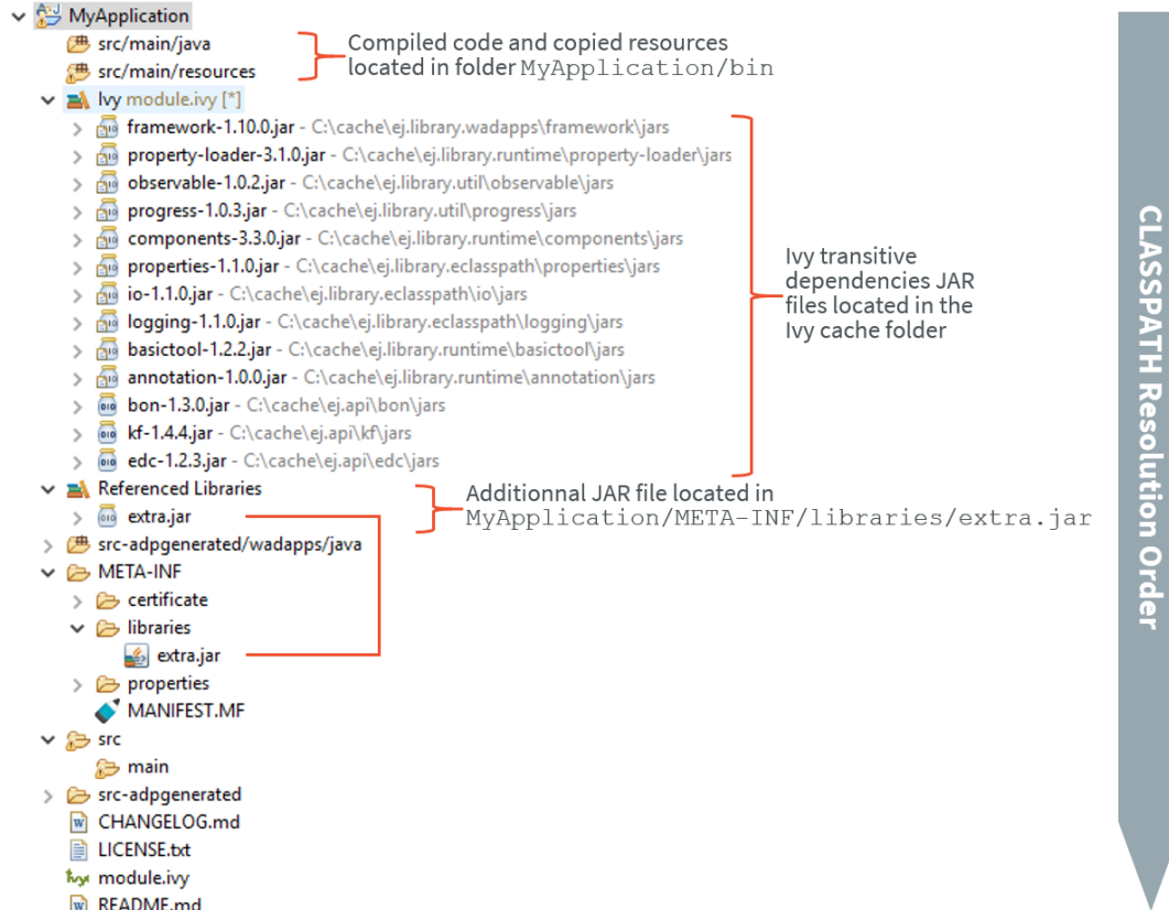
Fig. 29: MicroEJ Application Classpath Mapping
