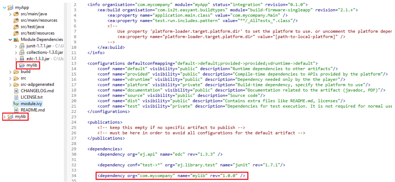
Fig. 35: A module and its dependency opened in the same workspace
