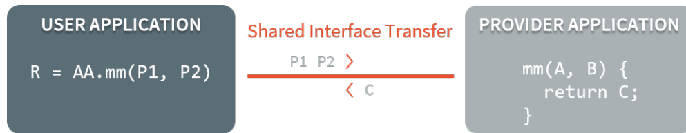
Fig. 23: Shared Interface Parameters Transfer
