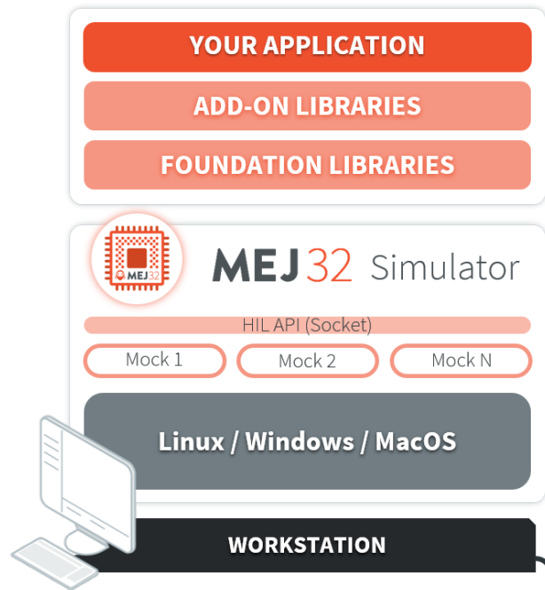
Fig. 48: The HIL Connects the MicroEJ Simulator to the Workstation.
