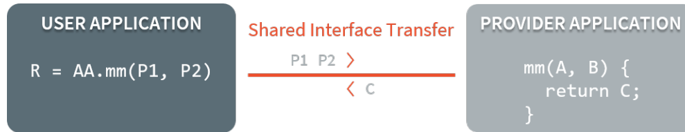
Fig. 23: Shared Interface Parameters Transfer
