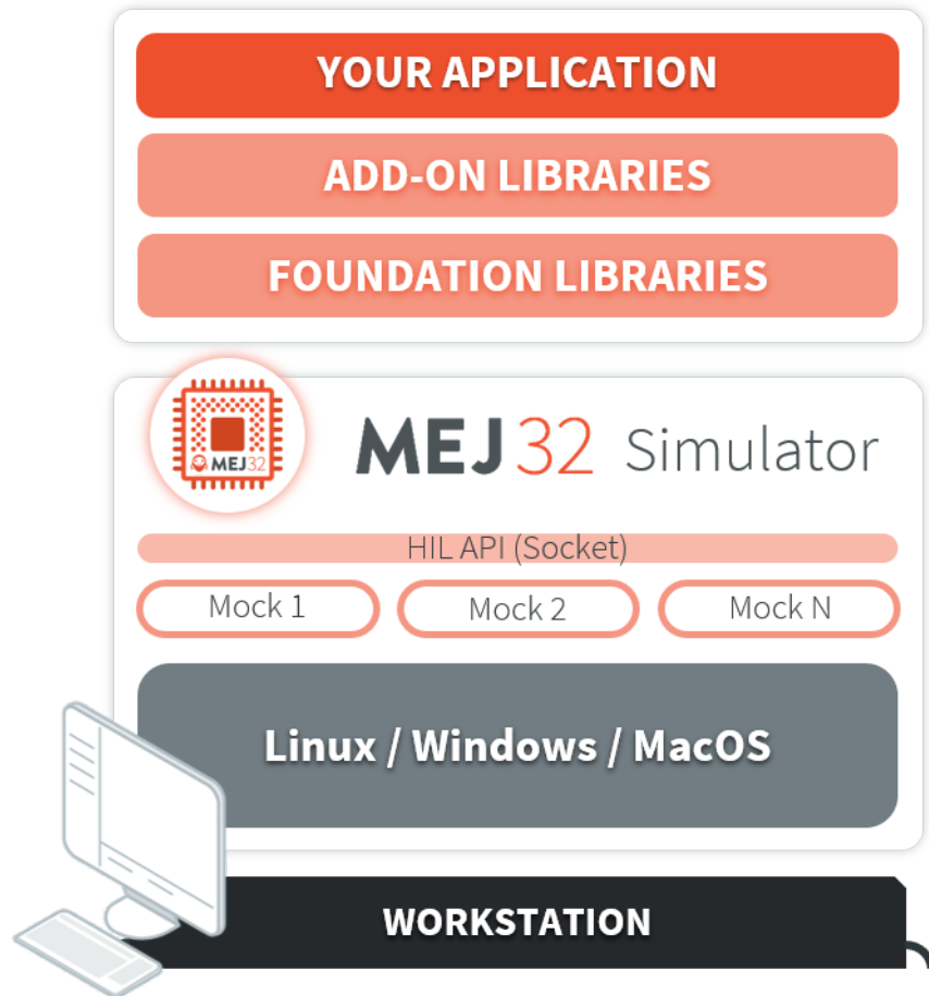
Fig. 43: The HIL Connects the MicroEJ Simulator to the Workstation.
