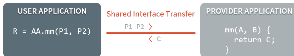
Fig. 17: Shared Interface Parameters Transfer
