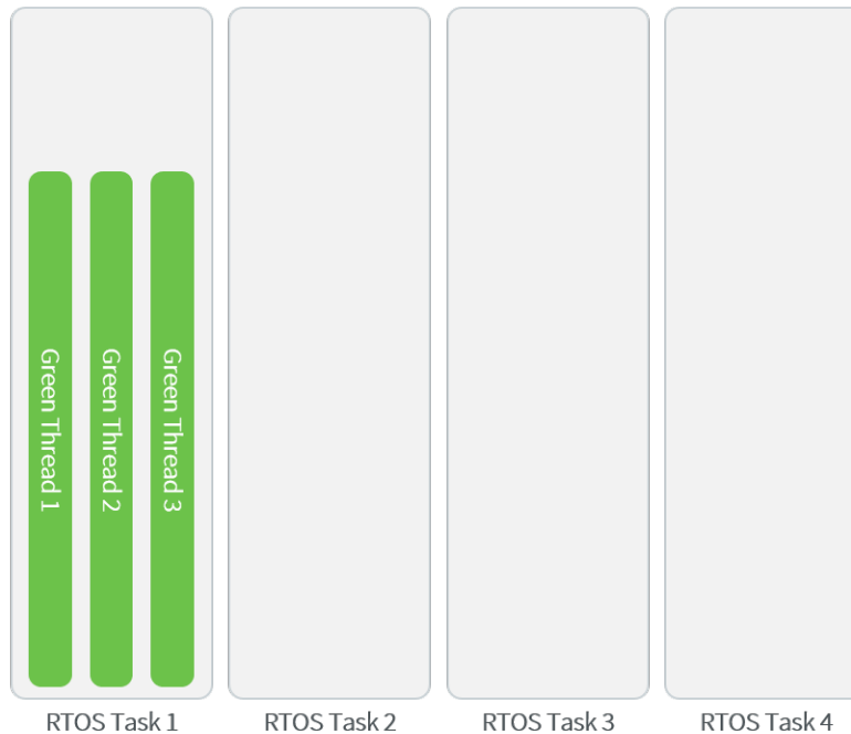
Fig. 18: A Green Threads Architecture Example
