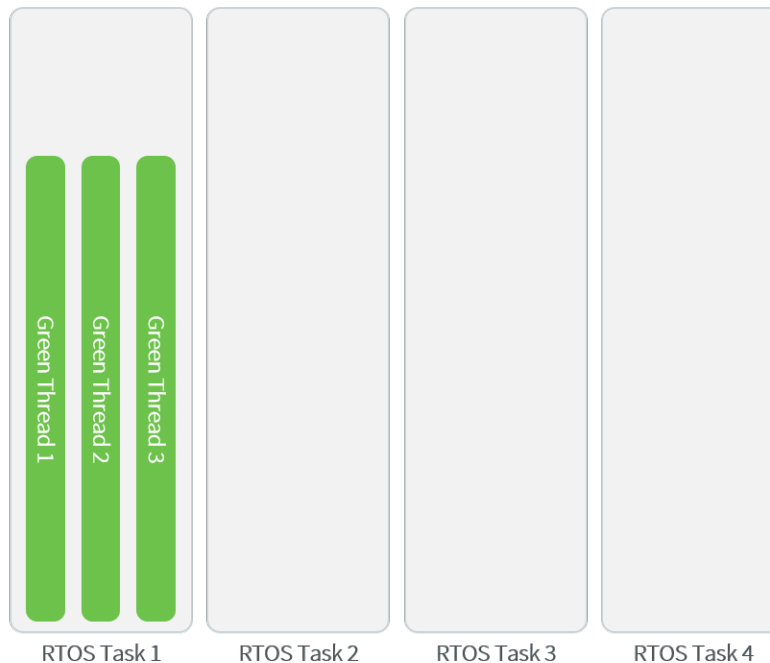
Fig. 16: A Green Threads Architecture Example
