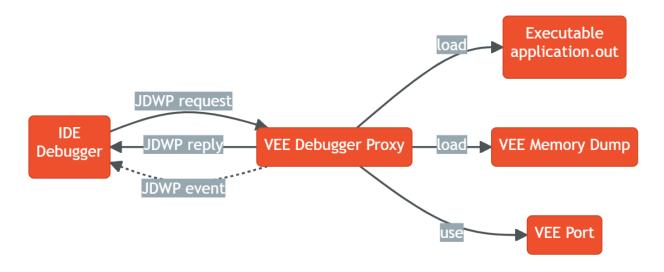
Fig. 36: Debugger Proxy Principle
