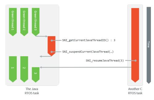
Fig. 31: Green Threads and RTOS Task Synchronization
