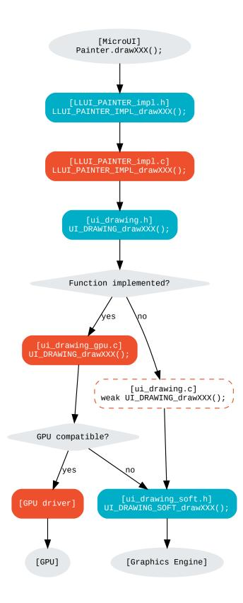
Take the same example as the default implementation (draw a line): the BSP just has to overwrite the weak function UI\_DRAWING\_drawLine :
