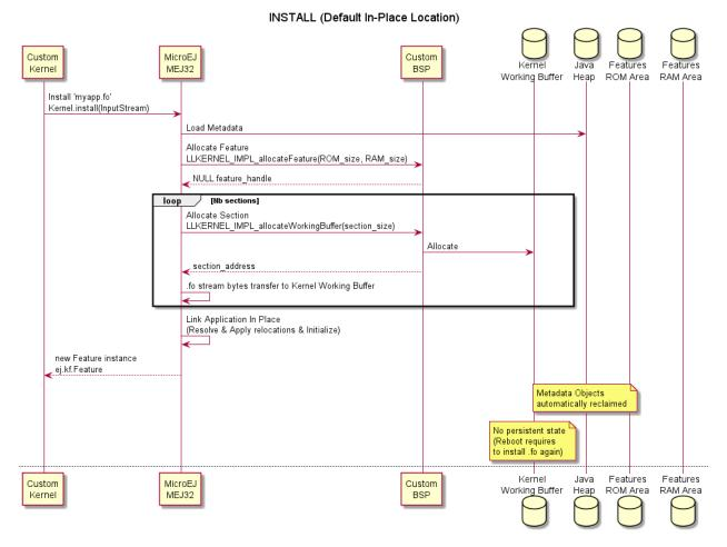
Fig. 28: In-Place Feature Installation Flow
