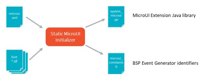
Fig. 42: Static MicroUI Initializer Process
