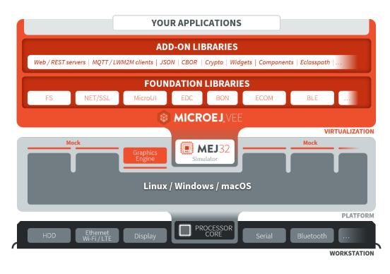
Fig. 3: MicroEJ Virtual Device Architecture
