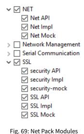
The Net API Module must be added to the *module.ivy* of the MicroEJ Application project to use the Net library.
