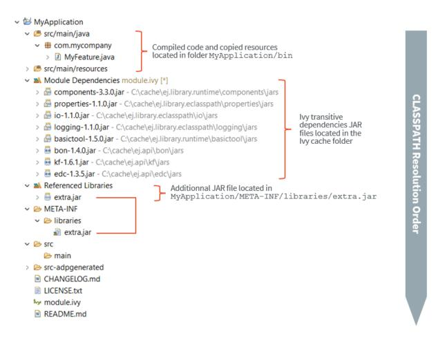
Fig. 4: MicroEJ Application Classpath Mapping
