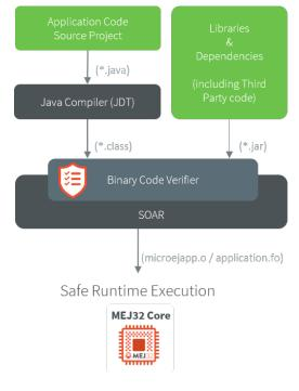
Fig. 1: Application Build Flow with Binary Code Verifier
