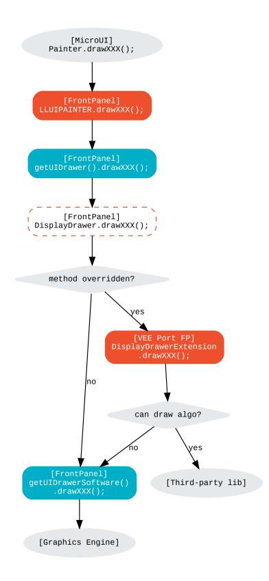
Let's use the same example as the previous section (draw line function): the Front Panel project has to create its drawer based on the default drawer:
