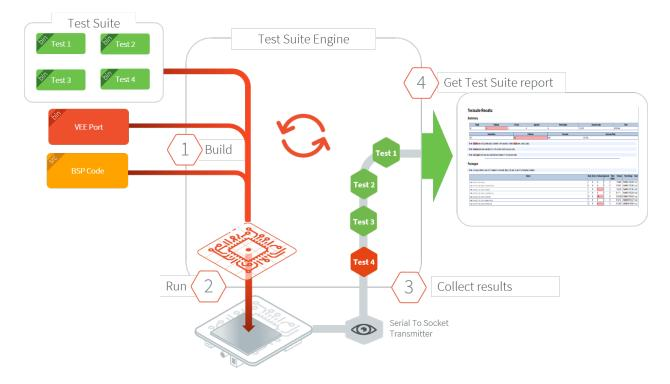
Fig. 16: VEE Port Test Suite on Device Overview
