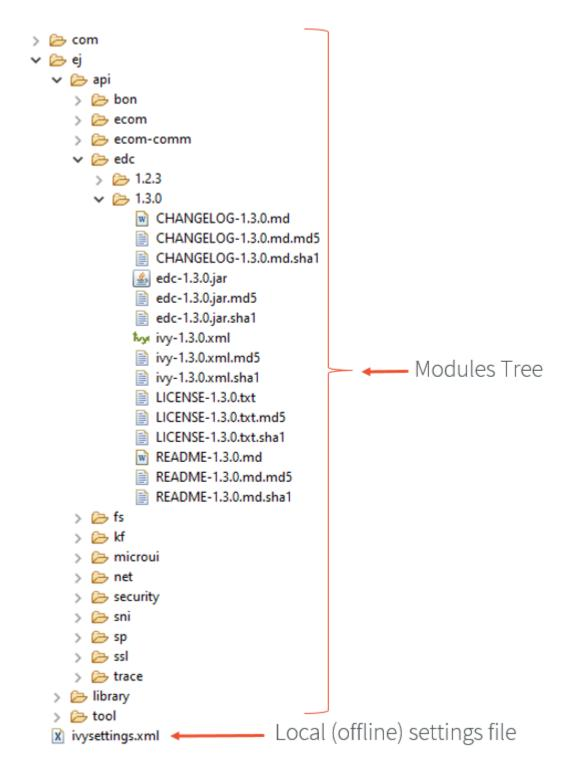
Fig. 51: Example of MicroEJ Module Repository Tree
