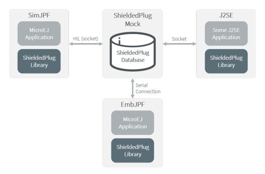
Fig. 77: Shielded Plug Mock General Architecture
