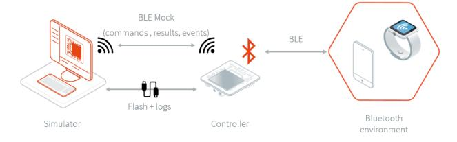
The Bluetooth LE mock controller is a hardware mock of the Bluetooth LE library. It means the Simulator uses a real Bluetooth LE device to scan other devices, advertise, discover services, connect, pair, etc... This design enables testing of apps in a real-world environment.
