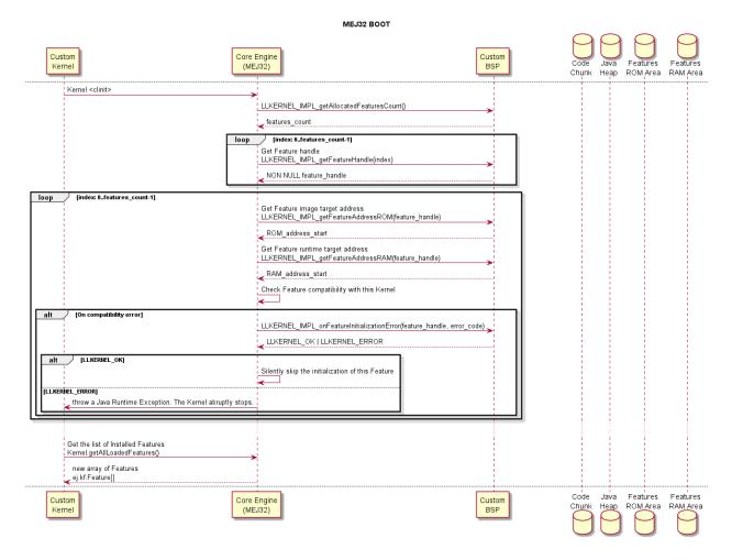
Fig. 26: Feature Installation Boot Flow
