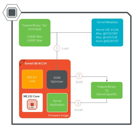
Fig. 12: Sandboxed Application Build on Device
