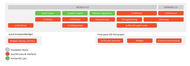
This set of classes and interfaces is available in the module com.microej.pack.ui#ui-pack. It offers the same capacity to override some built-in drawing algorithms (internal Graphics Engine drawing algorithms), to add some custom drawing algorithms, to manipulate the MicroUI concepts (GraphicsContext, Image, etc.) in the Front Panel project, etc.
