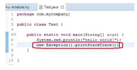
Fig. 67: Code to Dump a Stack Trace
