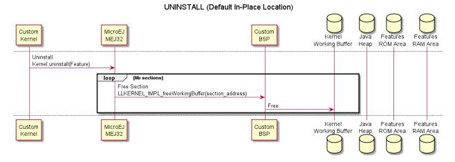
Fig. 29: In-Place Feature Uninstallation Flow
