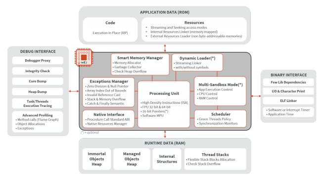
Fig. 18: Core Engine Block Diagram
