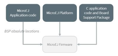
Fig. 11: MicroEJ Platform with no BSP connection
