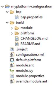
Fig. 8: MicroEJ Platform Configuration Project Skeleton
